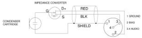
MICROPHONE WIRING DIAGRAM
